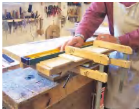
▲ Pic.31 The soundboard edges made true
